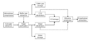
Figure 6: Baseline ISRU architecture for the initial Mars toehold, featuring oxygen and water acquisition by ISRU
