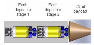
Figure 1: Earth departure stack with two 25 mt LOX / LH<sub>2</sub> propulsion stages per 25 mt payload
