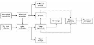
Figure 7: Alternative ISRU architecture for the initial Mars toehold with RWGS instead of zirconia electrolysis
