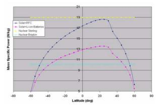
Figure 4: Results from equal-energy analysis of surface power system concepts as a function of Mars latitude
