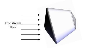
Figure 21: 70° sphere-cone aeroshell with L/D = 0.3  $(\alpha = 20^{\circ}, C_D = 1.40)$
