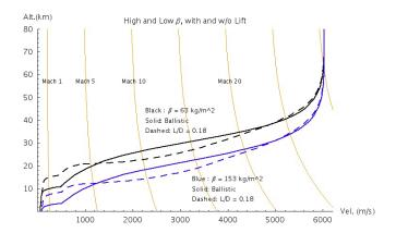
**Figure 11**: Ballistic and lifting (vertical L/D = 0.18) Mars EDL nominal trajectories for  $\beta = 63$  and 153 kg/m<sup>2</sup>.
