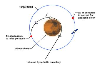
Figure 18: Mars aerocapture maneuver.
