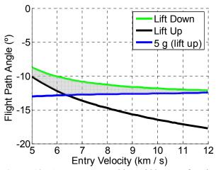
**Figure 19:** Aerocapture corridor width as a function of Mars entry velocity for an L/D = 0.3. With current navigation technology assumptions, an L/D of 0.3 is sufficient for Mars aerocapture.
