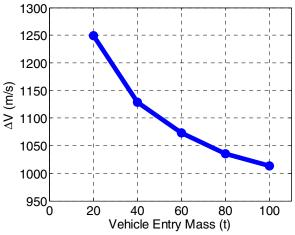
**Figure 22:**  $\Delta V$  for propulsive descent from Mach 3.
