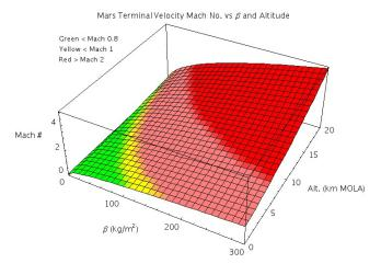
**Figure 3**: Terminal descent velocity comparison at Earth and Mars as a function of ballistic coefficient,  $\beta$ .
