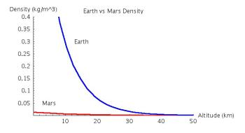
Figure 1: Earth and Mars atmospheric comparison.
