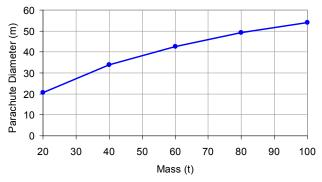
**Figure 24**: Parachute diameter as a function of entry mass for a parachute-assisted deceleration from Mach 3 to Mach 0.8 at an altitude of 2 km.
