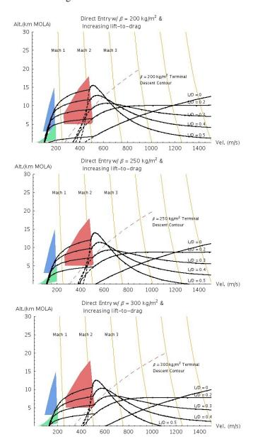
Figure 17: Increasing vertical lift for entry system with  $\beta = 200$ , 250 and 300 kg/m<sup>2</sup>.
