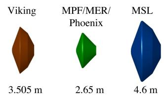
Figure 10: Viking-heritage 70-deg sphere-cone aeroshells.
