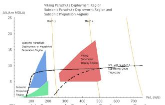
**Figure 14**: Supersonic Parachute Deployment Region, Subsonic Deployment Regions.
