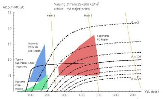
**Figure 15**: Increasing  $\beta$  from  $25 - 200 \text{ kg/m}^2$ .
