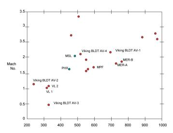
**Figure 13**: Mach and dynamic pressure history for all successful inflation disk gap band parachutes in Mars relevant conditions.
