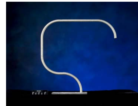
Thin-wall hollow tube produced by Lockheed Martin Tactical Aircraft Systems with laser Solid Freeform Fabrication process.
