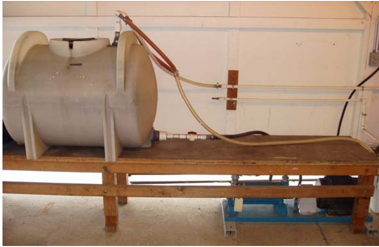
Figure 37. Water Cooling Pump and reservoir
