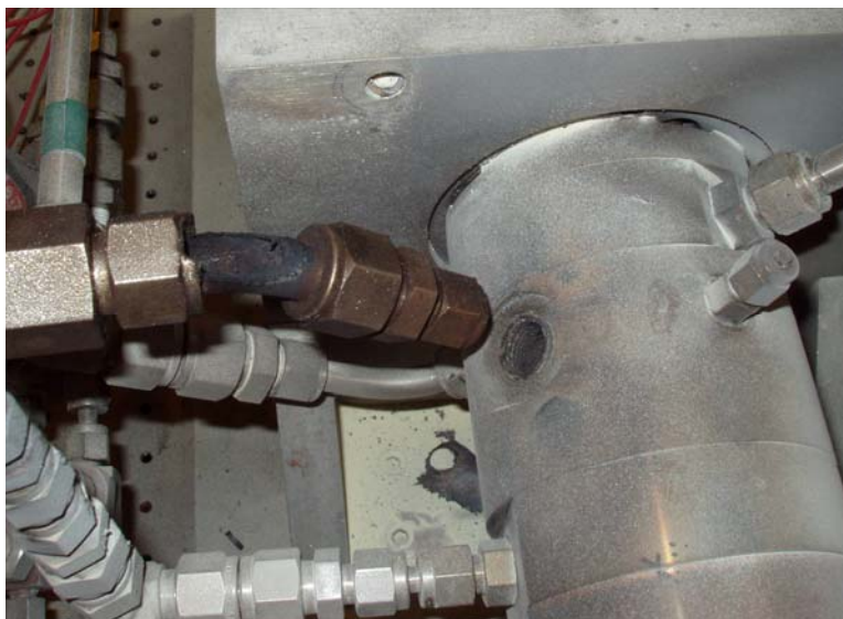
Figure 21. Burst Disk connection following the second hot fire test
