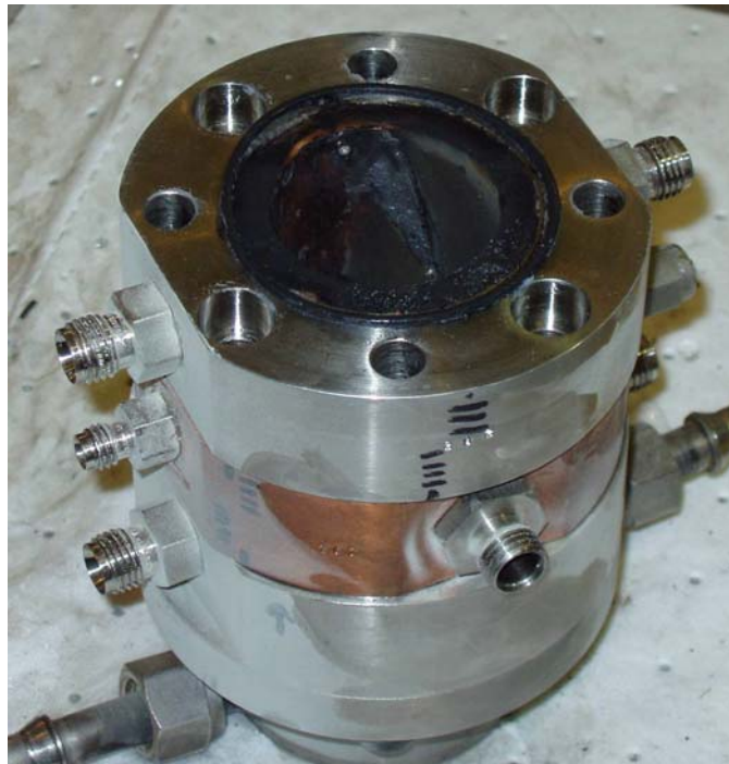
Figure 23. Combustion chamber filled with slag of retainer plates and glass beads following the second hot fire test
