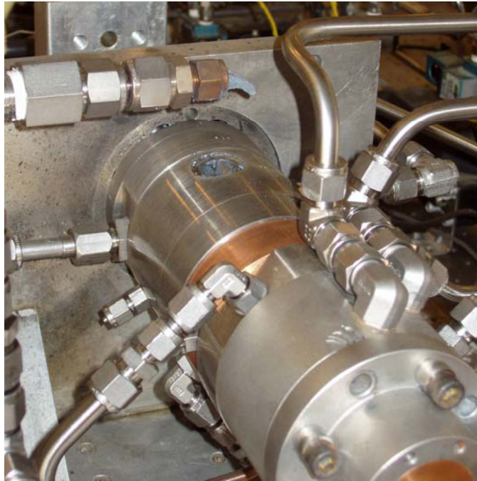
Figure 15. Premixed Injector following first test showing the burst disk blown with hardware loss
