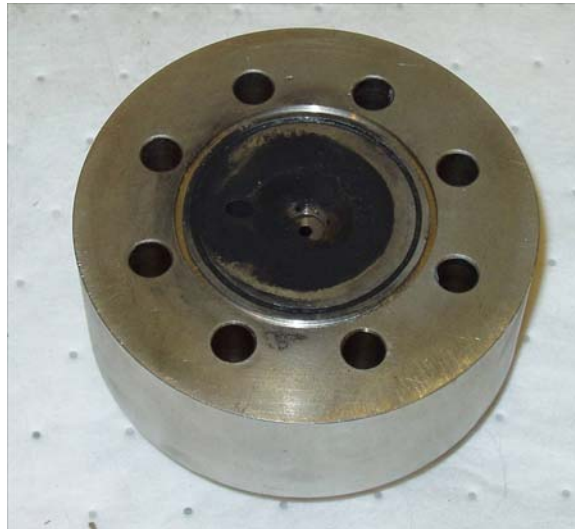
Figure 36. The Non-premixed injector with center post and two orifices impinging at 45 degrees
