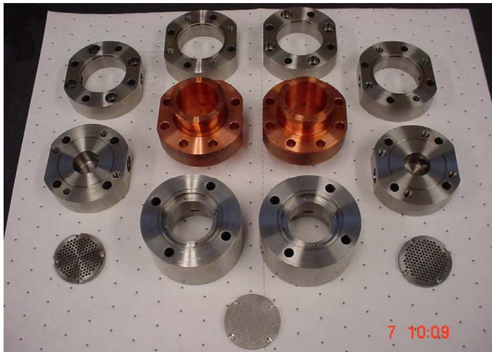
Figure 2. Sierra Engineering Machined Premixed Injector components 1
