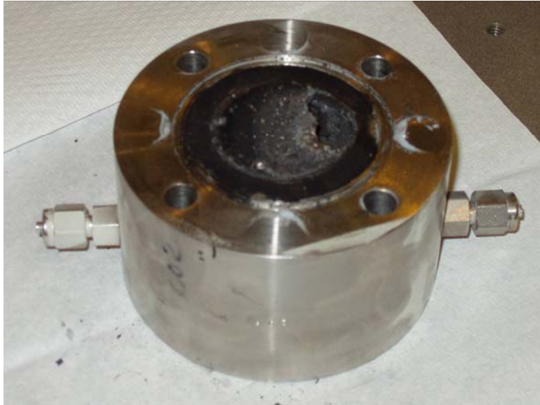
Figure 22. Injector plate following the second hot fire test
