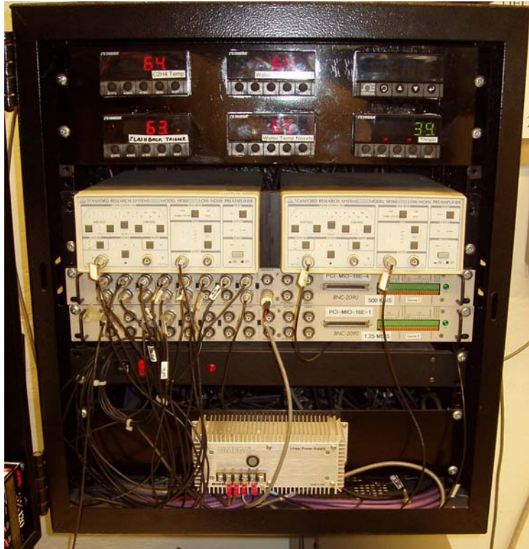
Figure 43. Test Cell Three Acquisition card and Omega Thermocouple meters
