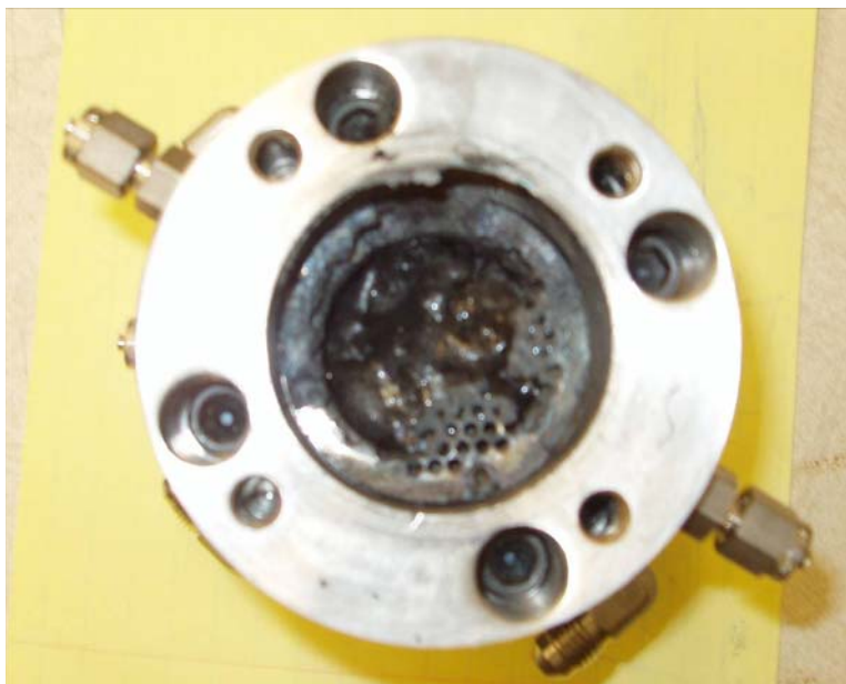
Figure 16. Premixed Injector showing the damage upstream of glass bead field
