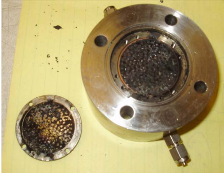
Figure 17. Premixed Injector showing the damage downstream of glass bead field and the orifice plate
