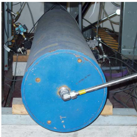
Figure 33. Accumulator for Ethylene Fuel
