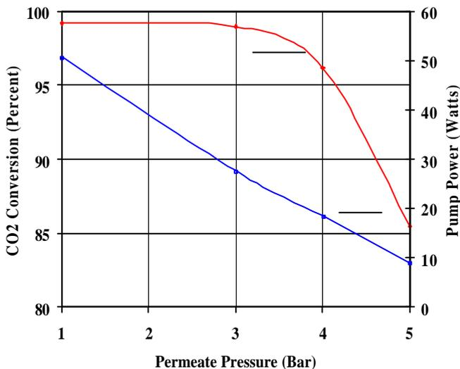
Fig. 5 Relationship between permeate pressure, CO<sub>2</sub> conversion, and pump power for RWGS with fixed membrane size.
