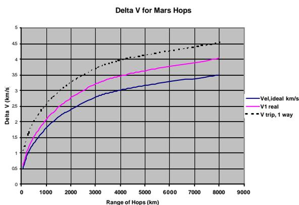
Fig 12. Delta-V required of Mars Hoppers as a Function of Range
