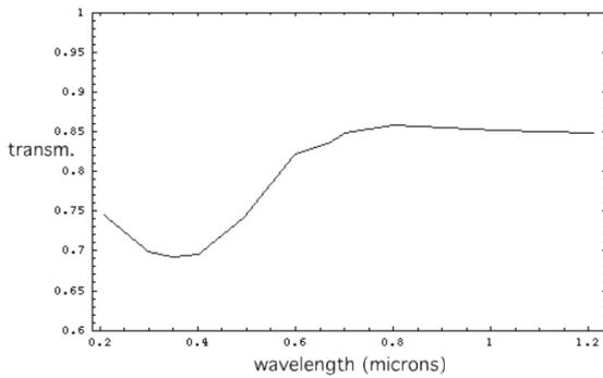
Figure 4.—Example Spectrum of Solar Energy as a Function of Wavelength on Mar, Modeled for the Case of Noon, Optical Depth  $\tau = 1$ ).
