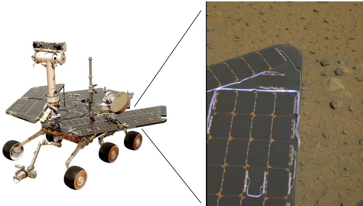
Figure 1.—Solar Array of the Mars Exploration Rover on Mars.
