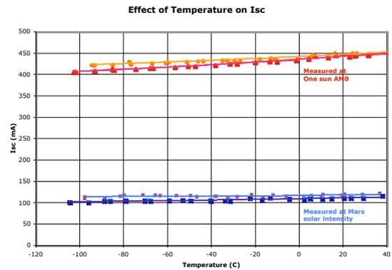
Figure 7.—Effect of Temperature on Cell Short-Circuit Current at AM0 Earth Solar Intensity (Top) and Mars Solar Intensity (Bottom).
