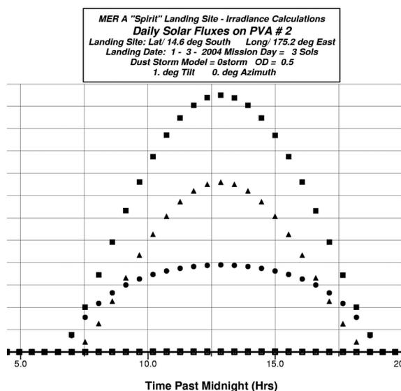
Figure 2.—The Diurnal Profile of Solar Energy on a Horizontal Surface on Mars (Low Dust Case,  $\tau = 0.5$ ), Showing The Direct (Circles), Scattered (Triangles), and Total Isolation During the Course of a Martian Sol.
